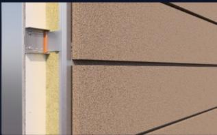
PCP takes planking profiles further. It uses a secret-fixed method like the IPP system but instead uses an extruded aluminium clip for structure engagement. As an open jointed system, it allows back ventilation, making PCP a true rainscreen. Horizontal installation is straightforward, starting from the bottom. PCP offers innovative design and aesthetics, making it an ideal solution.
