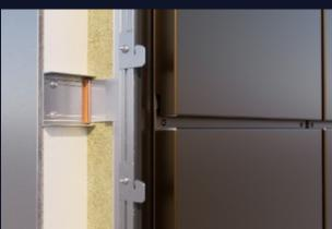
When a façade without visible fixings is demanded, a sensible solution is to use a secret-fix or 'hook-on' panel. As opposed to visible direct fixing through the panel and into the structure, SFC has its very own product-specific Helping Hand framing system. The framing is still simple to install but incorporates a hooked mullion which engages with the back of the panel, thus eliminating sometimes perceived unsightly panel fixings.
