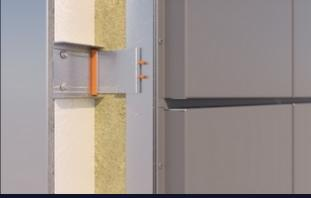
In contrast to TFP, DFC is a discreet-fix cassette panel designed to provide high performance, aesthetic appeal, and value. The panels are securely fixed within a shadow gap (typically 22mm), effectively concealing visible fixings. Similar to TFP, the supporting structure consists of a straightforward vertical or horizontal Helping Hand frame.
